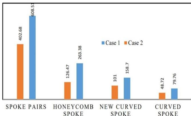
Figure 5: Comparison of vertical stiffness of the four tire models [12].
